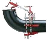
A clamp with the strength and ability to align and lightly reform pipes, the light weight design makes it easy to use. The feet of the clamp can be positioned equally around the chain to achieve an accurate pipe alignment in very little time.
